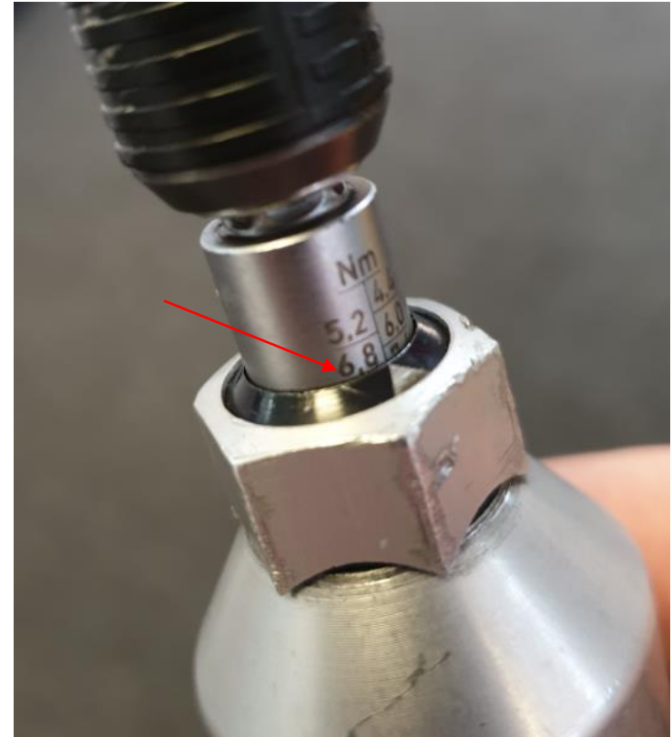
The correct torque setting is 6.8Nm
